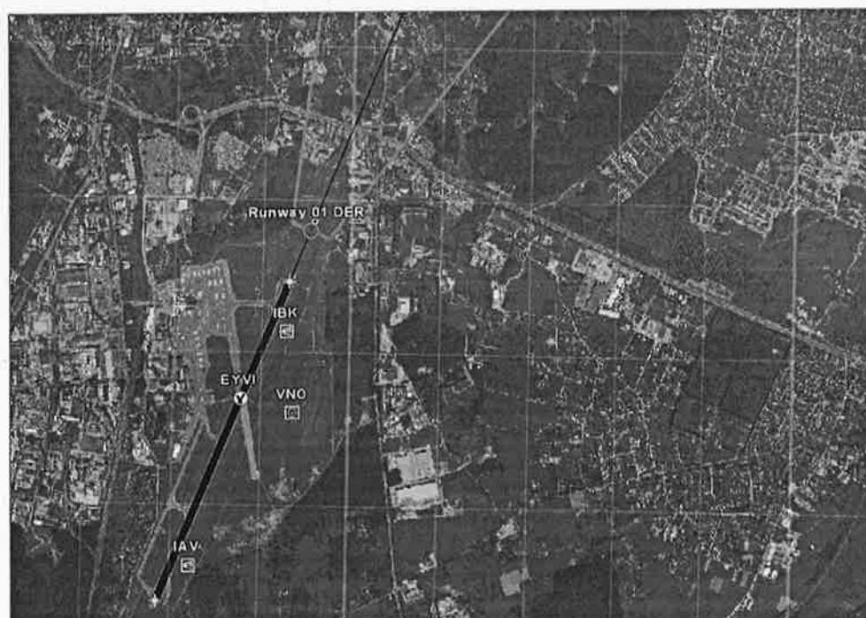
Figure 18: RWY 01 – Exemplary Obstacle Identification Surface
