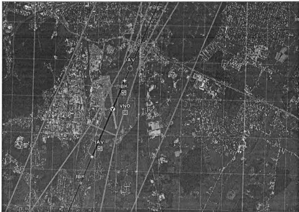
Figure 11: SBAS Approach – Exemplary Protection Areas
