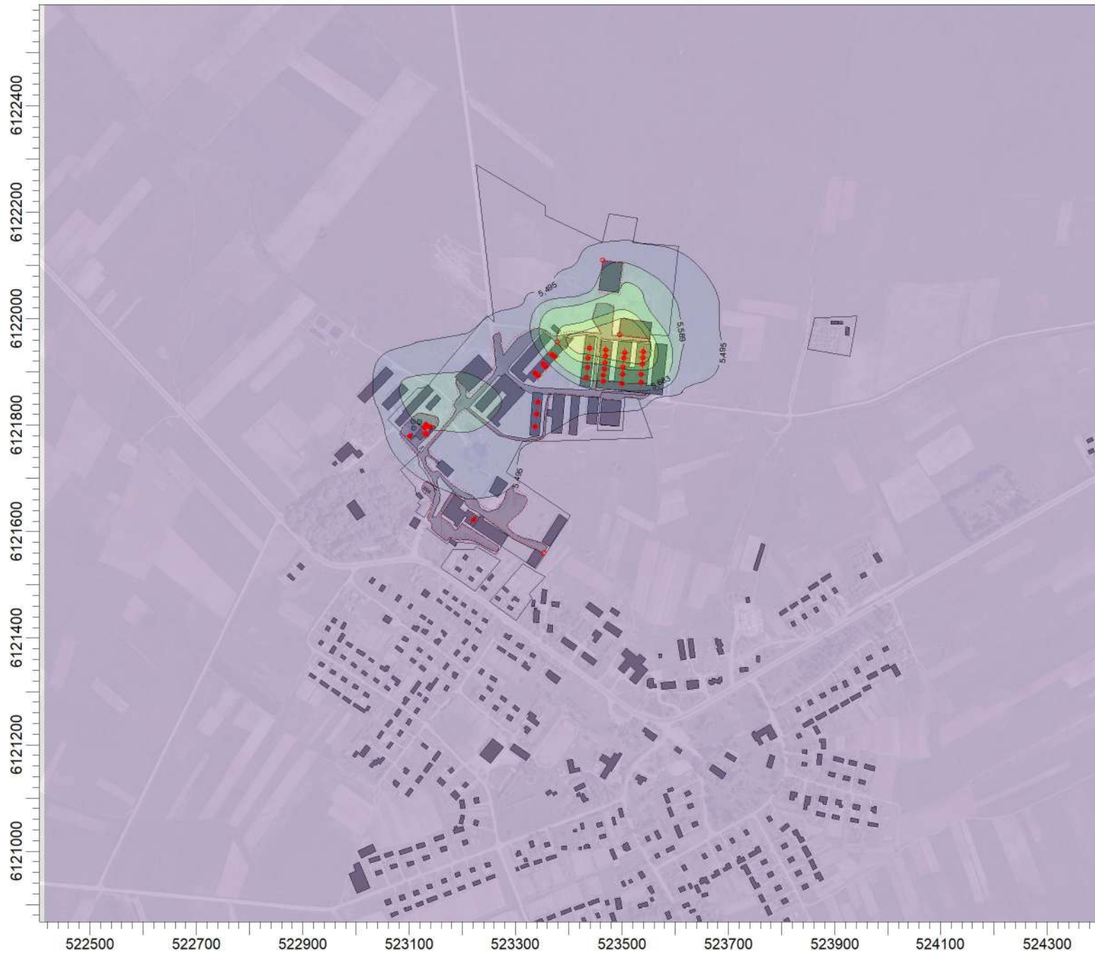
PLOT FILE OF ANNUAL VALUES AVERAGED ACROSS 5 YEARS FOR SOURCE GROUP: NO2 Max: 6,245 [ug/m^3] at (523514,75; 6121953,29)
