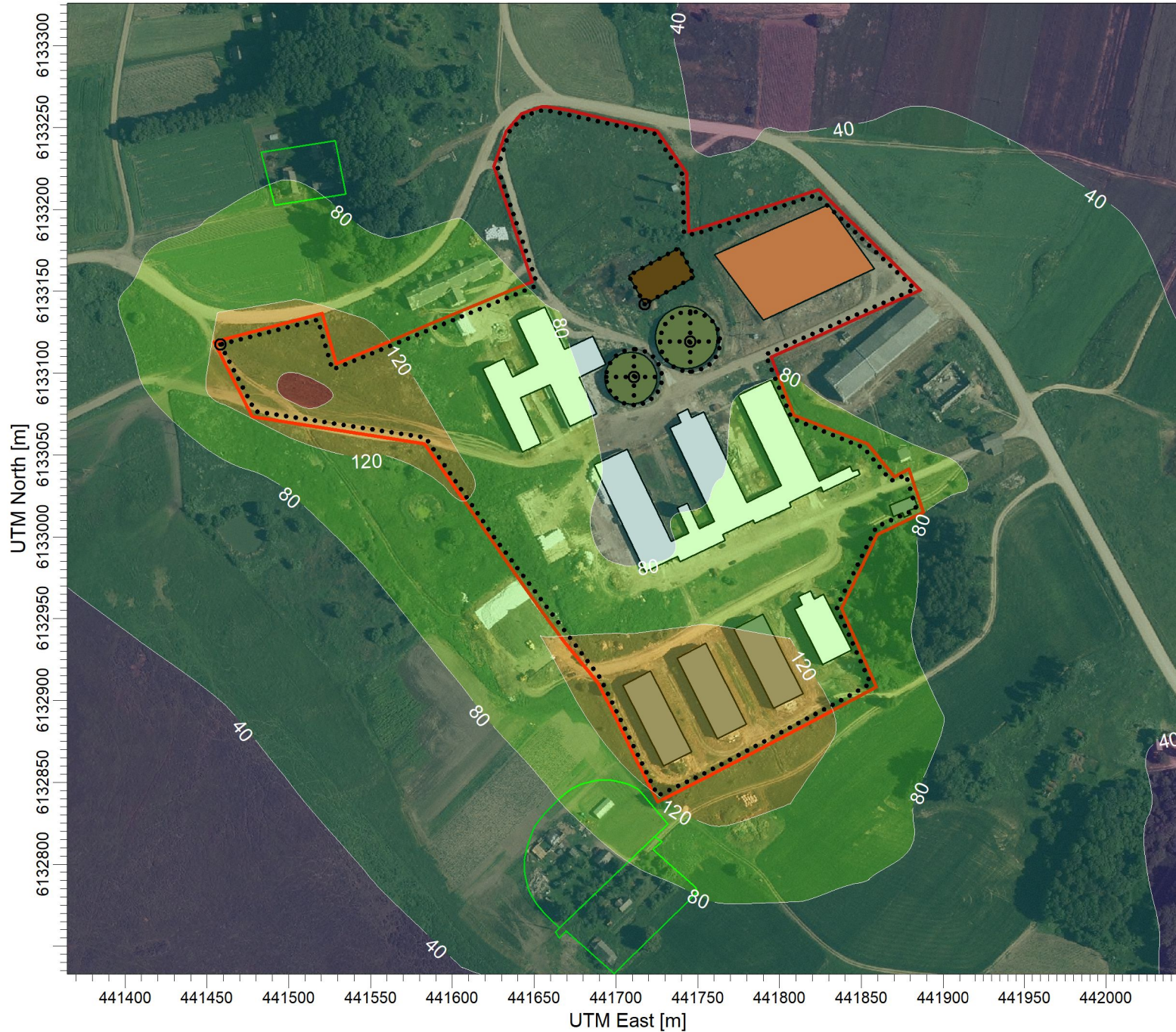
PLOT FILE OF 99.80TH PERCENTILE 1-HR VALUES FOR SOURCE GROUP: PŪV Max: 172,9 [ug/m^3] at (441505,99, 6133087,40)
