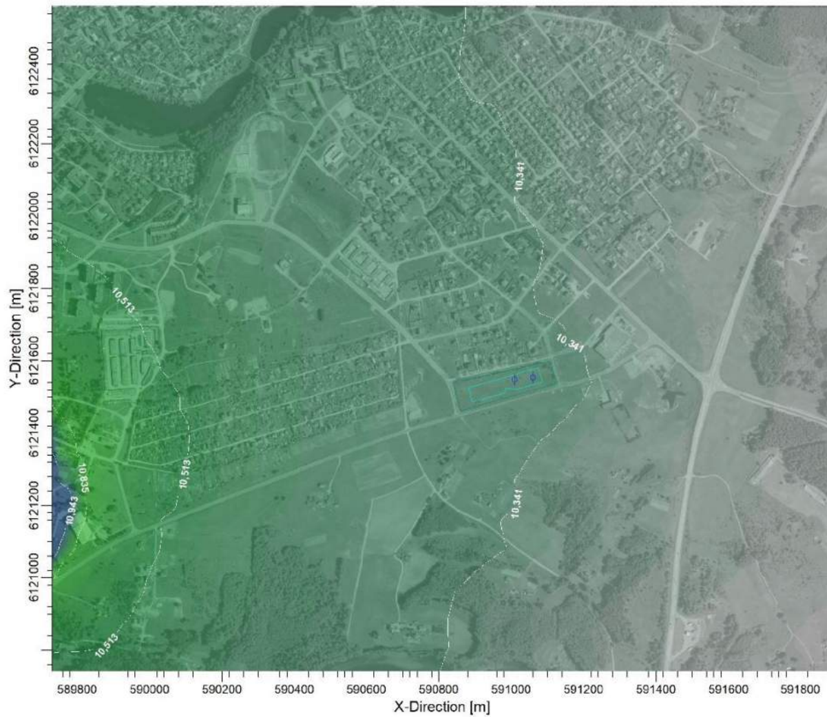
PLOT FILE OF 90.40TH PERCENTILE 24-HR VALUES FOR SOURCE GROUP: ALL Max: 18,48 [ug/m 3 ] at (589467,83, 6121148,84)
