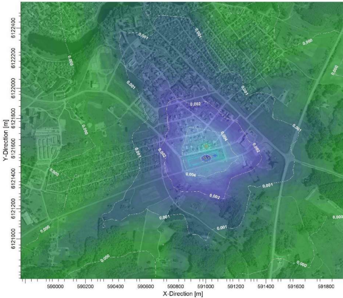
PLOT FILE OF HIGH 1ST HIGH 24-HR VALUES FOR SOURCE GROUP: ALL Max: 0.011 [ug/m 3 ] at (591005.59, 6121603.42)
