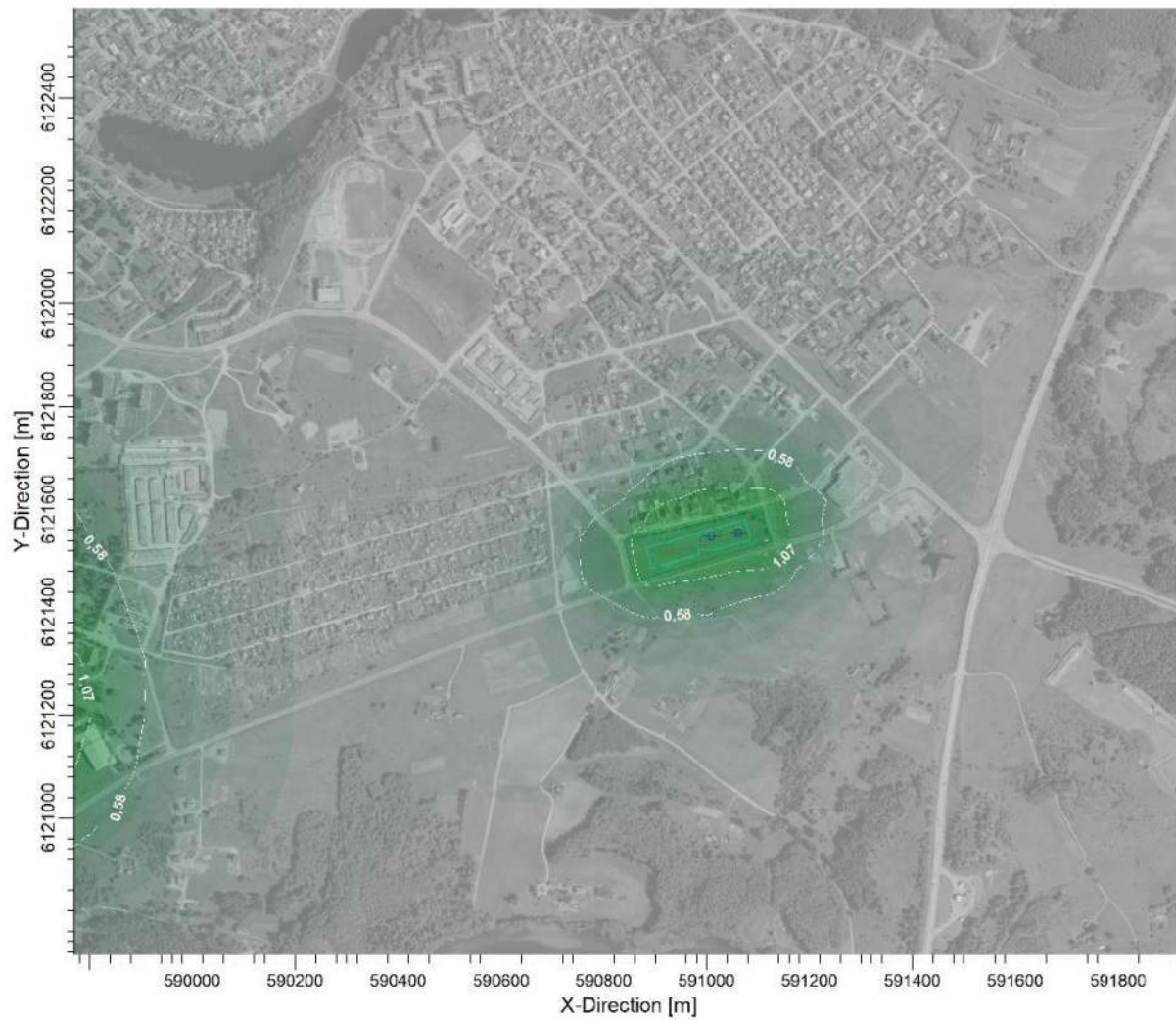
PLOT FILE OF 98.50TH PERCENTILE 1-HR VALUES FOR SOURCE GROUP: ALL Max: 12,25 [ \mu\text{g}/\text{m}^3 ] at (589467,83, 6121213,78)
