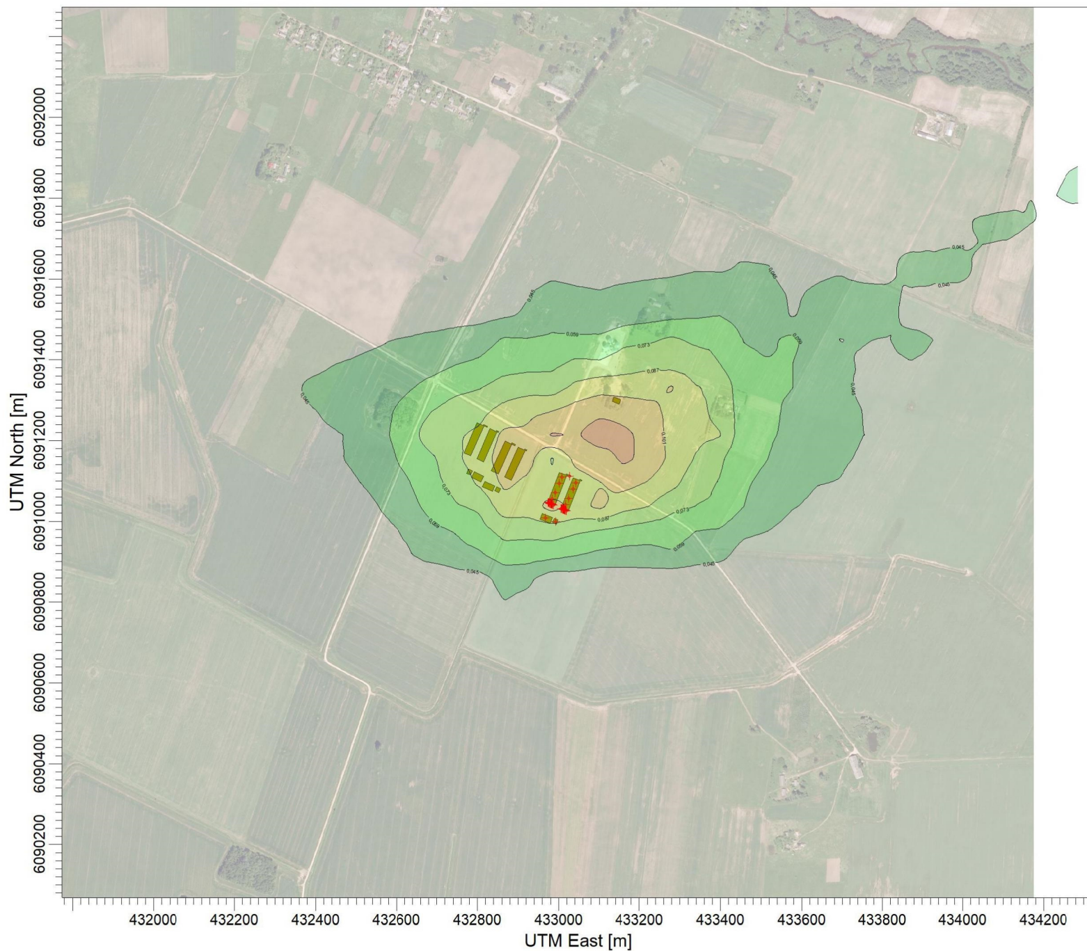
PLOT FILE OF 99.70TH PERCENTILE 1-HR VALUES FOR SOURCE GROUP: SOX Max: 0,129 [ug/m 3 ] at (433085,74, 6091230,22)
